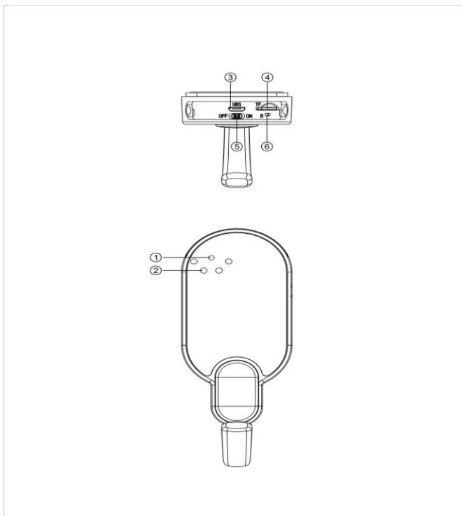
1.Camera lens 2.Night lights 3.USB charging output 4.TF card slot
