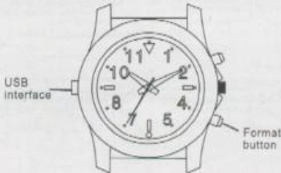
First, press and hold the format button to connect the data cable to the charger or the computer USB interface, this time the blue lights flashing is said to be formatted, when the blue light is bright when the format is completed. Because the memory card format is not right or the file is damaged, it can not be operated, please format it on the machine before it can be used normally.
